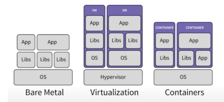
Containers, like VMs, isolate an application and its dependencies into a self-contained unit that can run anywhere.
